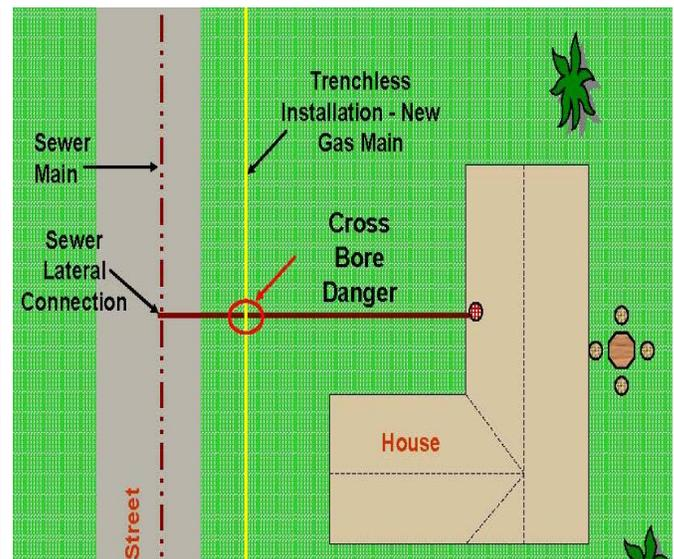
*A cross bore is defined as an intersection of an existing underground utility or underground structure by a second utility installed using trenchless technology resulting in direct contact between the transactions of the utilities compromising the integrity of either utility or underground structure.*
