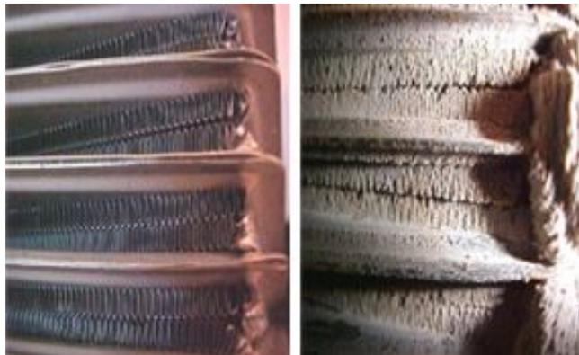
*Evidence of siloxanes in biomethane is found in the form of a white powder in the hot sections of gas turbine components, as a light coating on various types of heat exchangers, in deposits on combustion surfaces in reciprocating engines, and as a light coating on post-combustion catalysts.*
