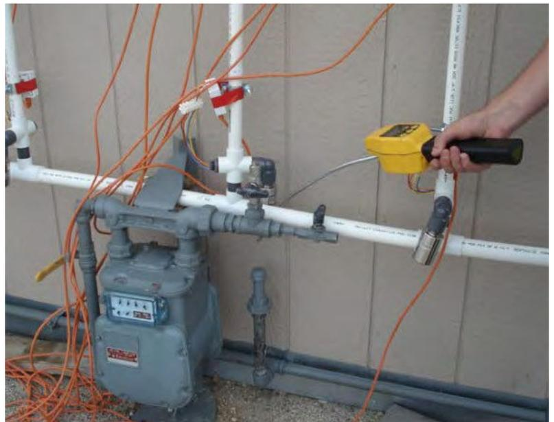
performed in an outdoor building at the Gas Technology Institute testing facility. An array of gas sensors were used to monitor gas concentrations from 0% to 100% gas at 15-inch intervals and at various locations around the leak source.
