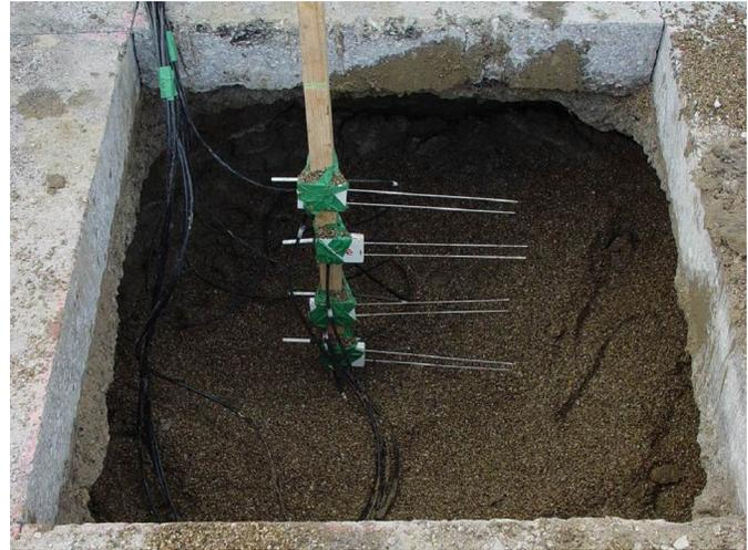
**Moisture and temperature instrumentation in a bellhole.**
