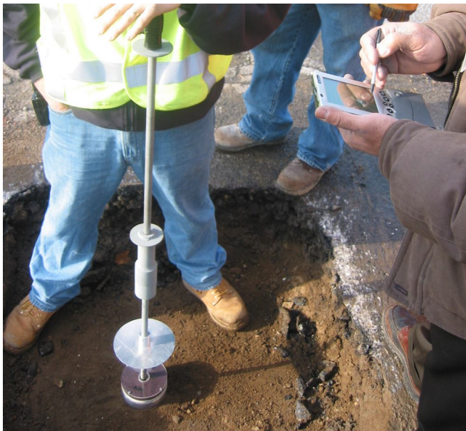
Research has shown the Utility Dynamic Cone Penetrometer to be an attractive, cost-saving alternative to more commonly used soil-compaction-measurement equipment.
