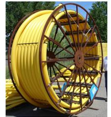
Since 1997, Gas Technology Institute has been investigating a similar product — Polyamide 11 (PA11) — for use at higher pressures, demonstrating the ability of two-inch-diameter PA11 pipe to operate safely at a pressure of 200 psig. Based on successful testing, program sponsors expanded its R&D initiative to other potential piping materials.
