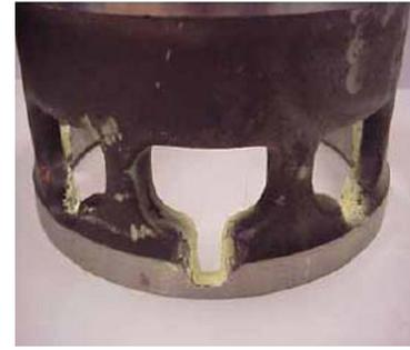
**Control valve cage with elemental sulfur deposition.**
