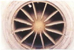
Deposits of “elemental sulfur” – which can block natural gas pipes and equipment – is becoming an increasing concern in the natural gas industry. As a consequence, research was conducted to develop a better understanding of the sources, causes, and mitigation possibilities for sulfur deposits found in gas operations.
